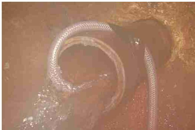
Figure A.9: The sampling tube was telescoped into the discharge pipe at Afra spring.
