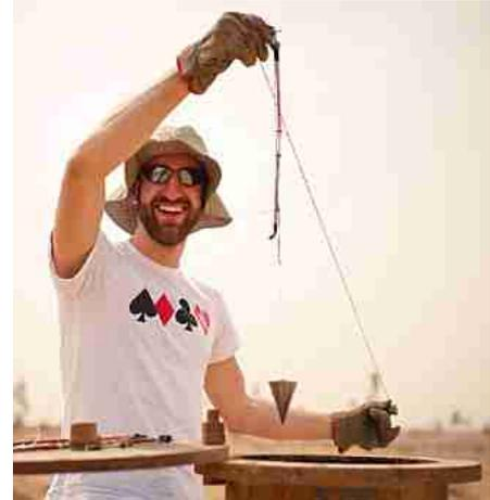
(b) Lowering the deepest diffusion sampler, an additional weight is attached.
