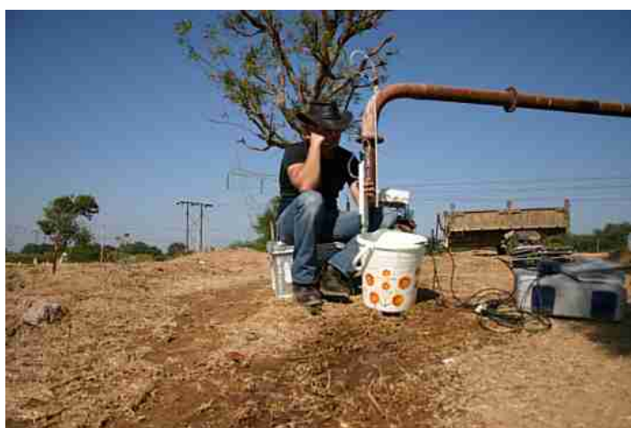
Figure 3.8.: Picture of a sampling at an Indian irrigation well. Tubes are connected to the air outlet of the pipe.
