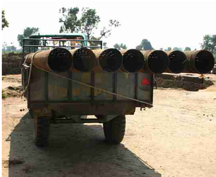
Figure 3.4.: Picture of the used pipes for the well's screen.
