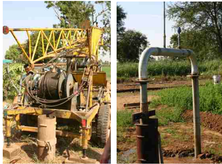
(a) A groundwater well drilling site. (b) A typical agricultural well of Gujarat.
