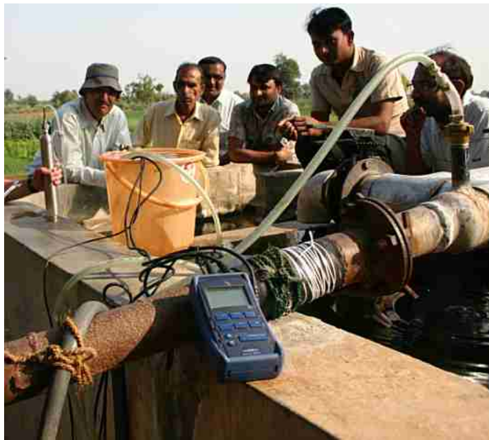
Figure 4.1.: Picture of the WTW water probe in use. Sensors measure groundwater collected in a flushed bucket. The brass connectors used to attach tubes to the air outlet are shown on the right.
