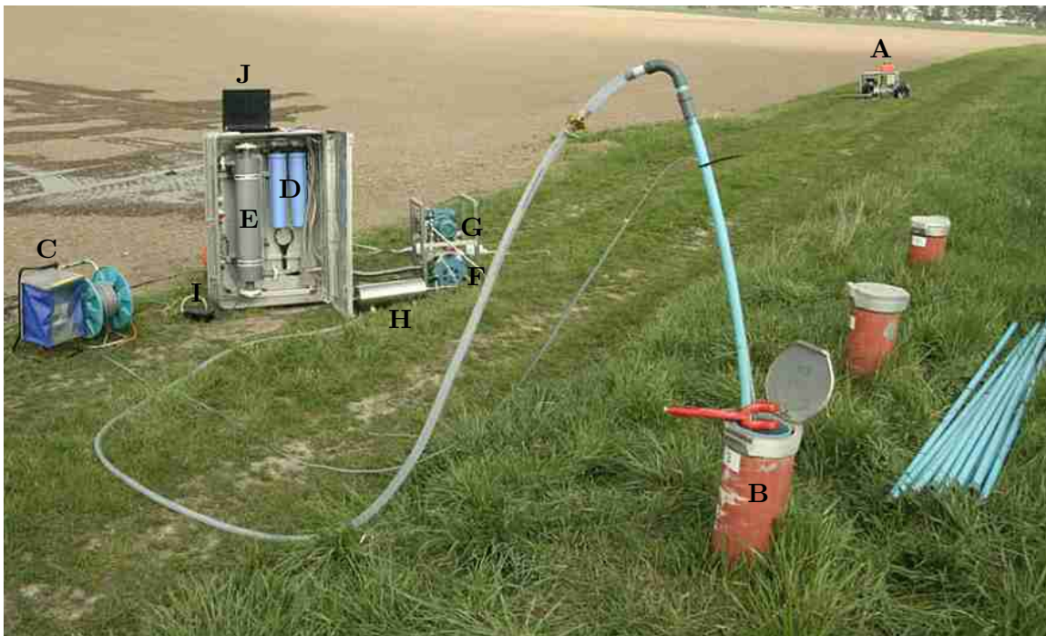
Figure 3.1: The final setup for water degassing during a field trip, which is supplied with power by the alternating current generator (A). The water pump MP1, submersed in the well (B), is controlled by an adjustable converter (C). The water is pumped through the water filters (D) and degassed by the membrane contactor (E). The outlet of the vacuum pump (F) is connected with the compressor (G), which compresses the gas in the sample cylinder (H) to a pressure of up to 7 bar. Control parameters are read out by an analog to digital converter (I) and displayed with LabView software on a laptop (J).
