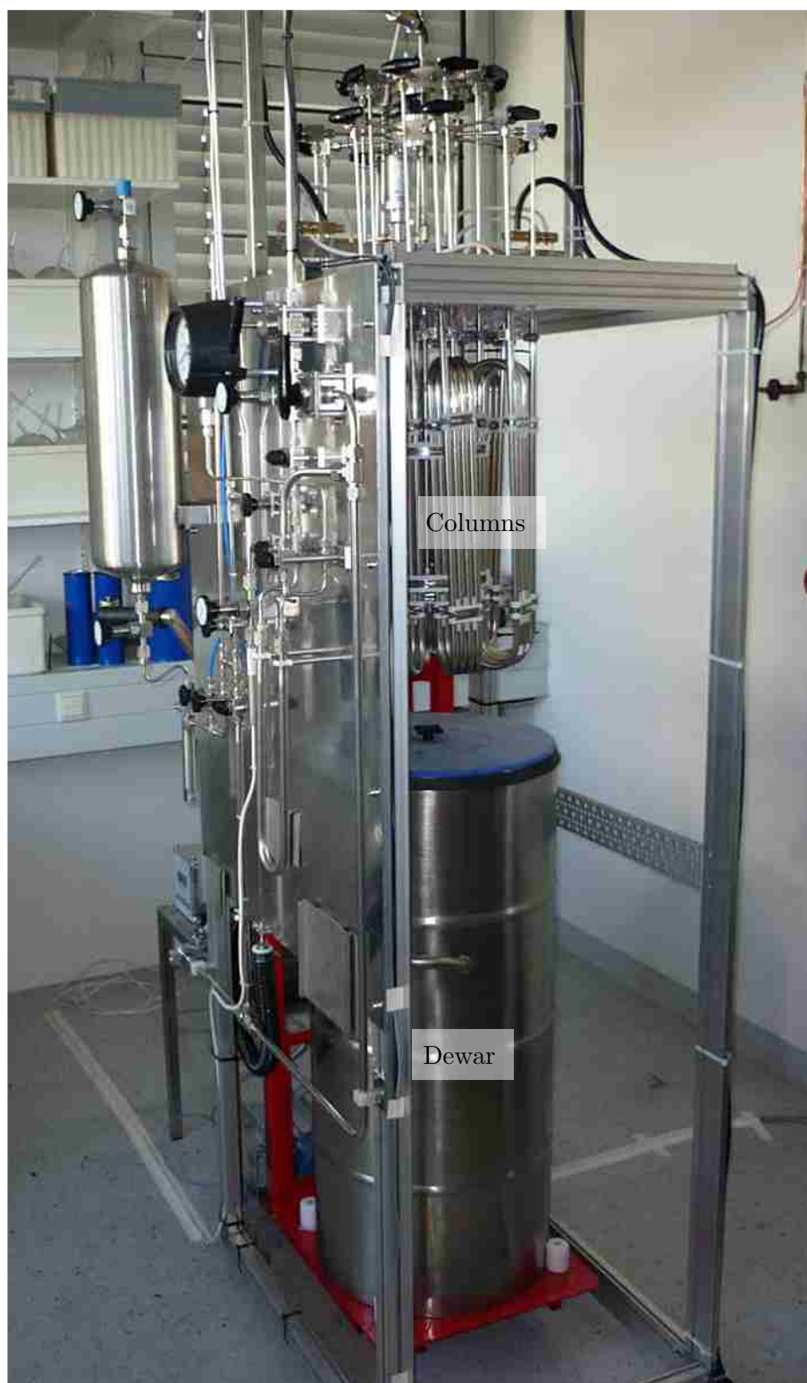
Figure 4.3: The setup for argon separation. During the separation, the dewar partly filled with liquid nitrogen is lifted in the upper position, insulating thermally and cooling the zeolite columns with a swirled, cold nitrogen atmosphere. When the columns are heated for regeneration, the dewar is moved back into the lower position as shown on the figure.
