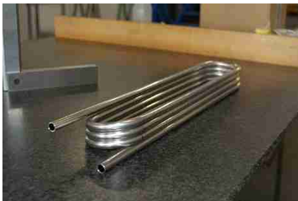
Figure 4.2: One of the nine columns before installation. The length of the column as it can be seen here is 528 mm, while the length before bending is 4229 mm. The inner and outer diameter of the tubing are 10 mm and 12 mm, respectively. Photo by [Dockweiler AG., 2009].
