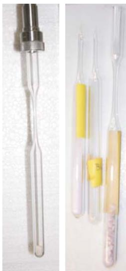
**Figure 3.23:** Glass vials for microwave extraction. On the left side a vial including a speleothem sample is displayed, which is attached to the preparation system using an o-ring connection. On the right side two pumped and by flame-sealing closed vials as well as one original glass vial are shown.
