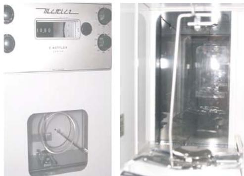
**Figure 3.7:** High precision balance (Mettler Toledo) with a precision of 2  $\mu\text{g}$ . The sample is put on the small roundish dish inside a chamber which is protected from air motion by sliding windows.
