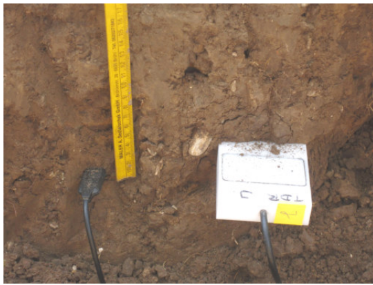
(a) Installation of sampling probes at the sampling site near Mannheim: FDR (left) and TDR (right).
