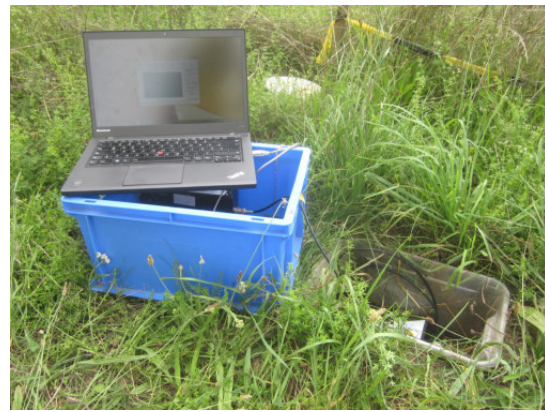
(b) Record of a TDR trace at the sampling site by means of a laptop and a high frequency generator.
