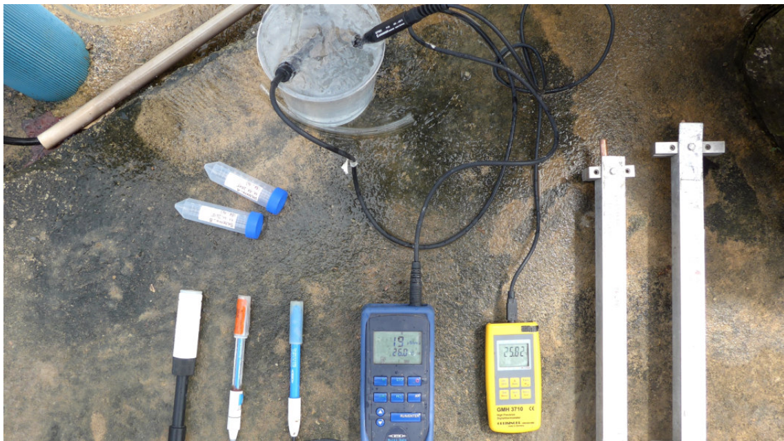
Figure 3.4: Groundwater sampling during the field campaign in Brazil. From right to left: copper tubes on aluminum racks for NG analysis; Greisinger GMH3710 thermometer (yellow device); WTW Multi 340i (blue device) with sensors for pH value, ORP value and dissolved oxygen content; the conductivity sensor is inserted into the bucket. Bottles for tritium and stable isotope analysis are situated above the sensors.
