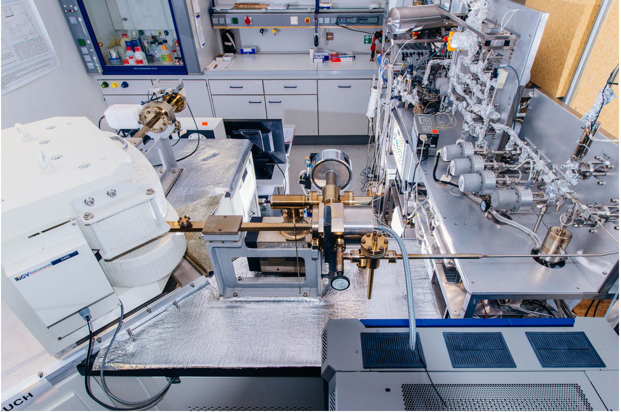
Figure 5.1: The mass spectrometry laboratory at the Institute of Environmental Physics at Heidelberg University . On the right is the extraction line built by Friedrich [2007], leading through a thin steel tube towards the ion source in the center of the image. On the left hand side, the flight tube and the magnet of the GV5400 are visible.
