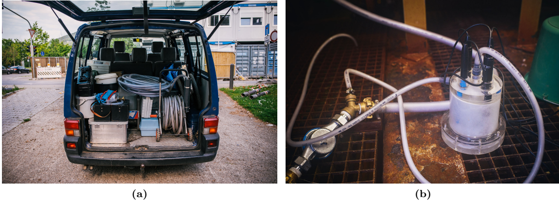
Figure 4.3: (a) The sampling gear required for all of the TRACE study’s participants, fitting into a small VW bus. (b) The WTW MultiLine probes during inline measurement at thermal well MM (the amount of bubble formation is the most extreme witnessed by the author in six years of groundwater sampling, an absolutely exceptional occurrence).
